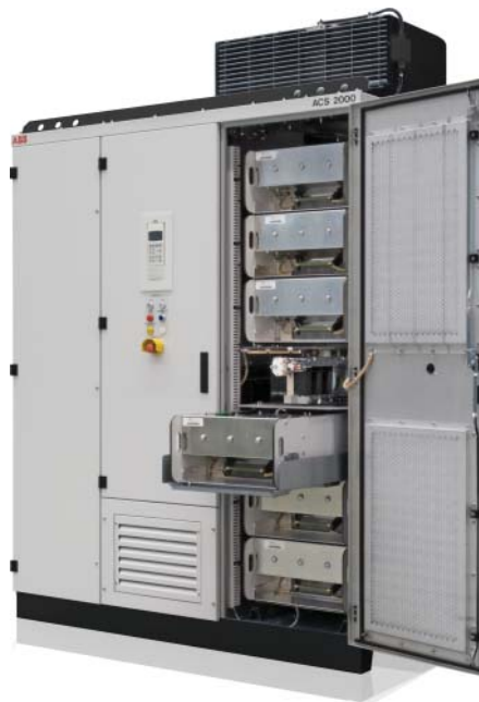
Figure 13.15 Five-level ANPC inverter with a rated voltage of up to 6.6 kV and a rated current of 98 A. The three phase models of the inverter and of the active front end, respectively, are shown on the right-hand side. Source: ABB Image Bank. Reproduced with permission of ABB Ltd
